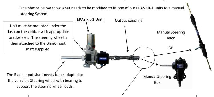
Output Coupling needs to be adapted the manual steering unit. Modify the input shaft of the manual steering box or steering rack. Via an adaptor or machine a 14mm A/F section on the shaft to take the lower Coupling clamping design as per photos below.
