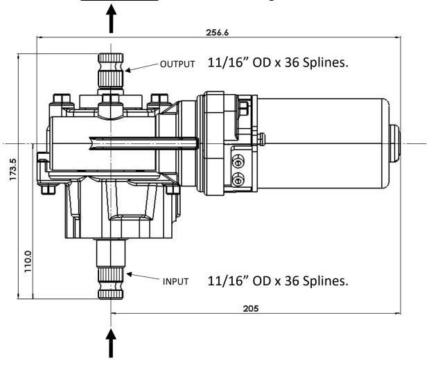
Input Shaft from Steering Wheel via driver to Unit.
