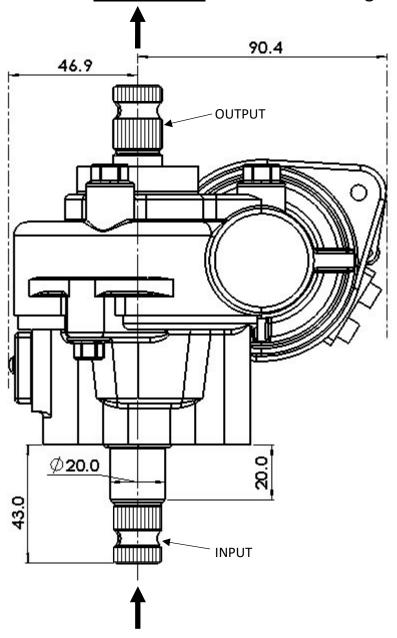
Input Shaft from Steering Wheel via driver to Unit.
