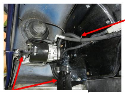
This Pump has a remote reservoir and the supply / return hoses are clamped to the chassis rail for extra clearance. The reservoir was mounted inside the engine bay.
