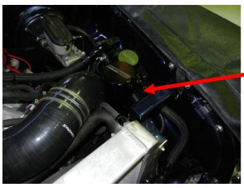
Hoses going through inner guard to Supply the pump with fluid & Return Hose from Steering Box to reservoir.
