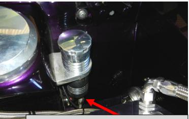
Reservoir Hoses plumed through inner guard -Supply to pump & Return from Steering Rack.
