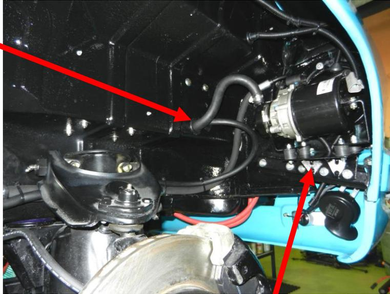
Brackets were made to mount Pump to Front of the RHS Inner-guard.
