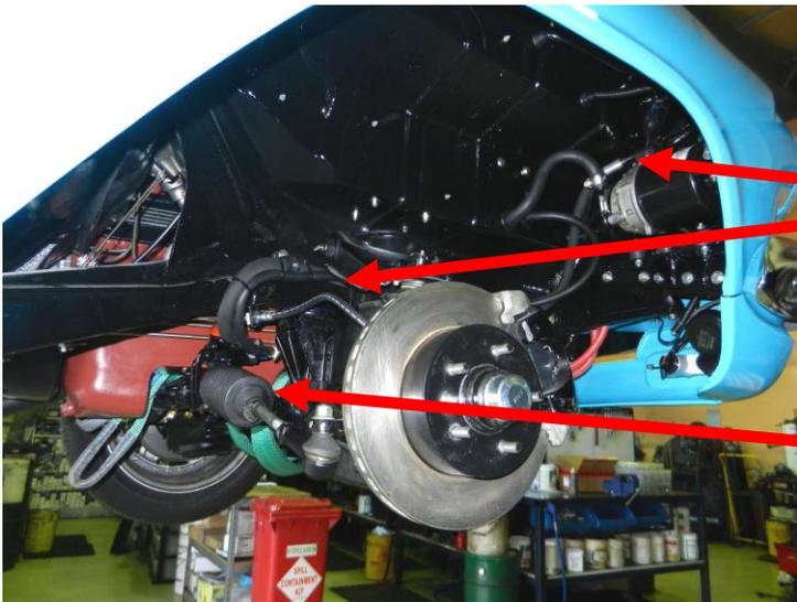
High-Pressure and return lines made for fit, running along the chassis rail.
