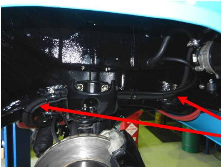
Electric Pump Mounted to Front of the Inner-guard.
