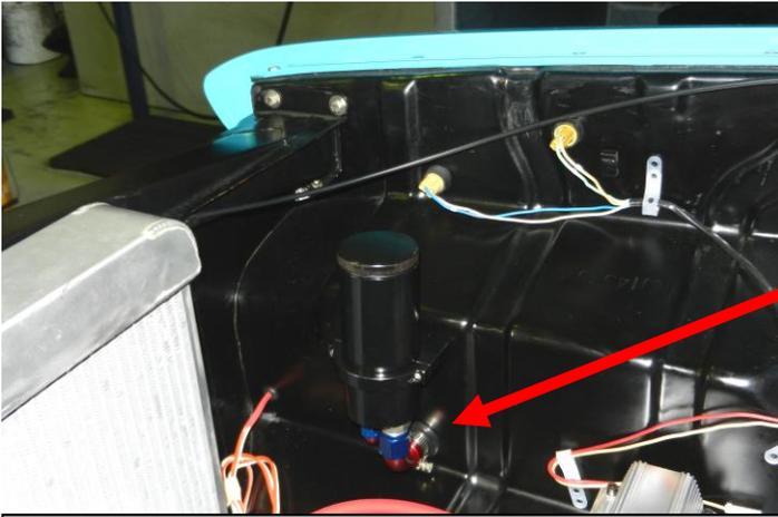
Hoses going through inner guard to Supply the pump with fluid & Return Hose from Steering Rack to reservoir.
