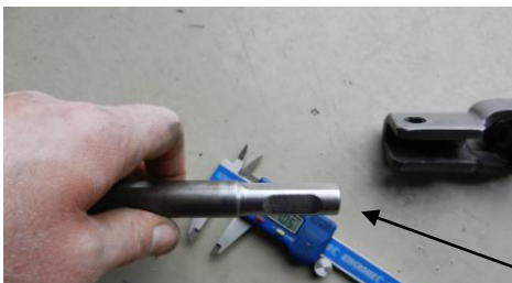
14mm A/F section on input shaft to fit lower output coupling.
