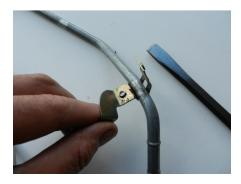
3. Fit the support bracket, use the bolt & nut. Bolt bracket to new hose.
