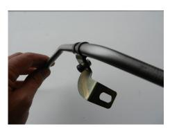
4. Finished photo showing support bracket bolted to new hose-17, ready to be fitted to the vehicle.
