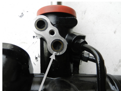
Install the NEW "Duck Bill Seal" into the Lower Rack port.
