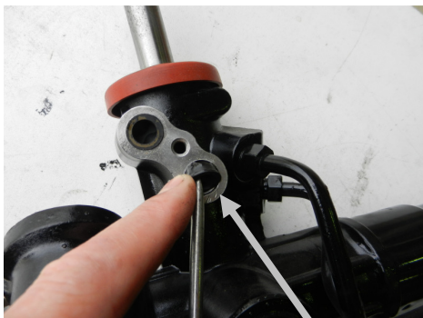
Using a screwdriver gently pry the OLD "Duck Bill Seal" from the Rack port.
