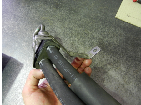
With the tag unclipped gently open the outer steel bracket and remove. Take-care not to over bend the bracket.
