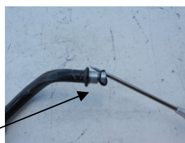
Use a scriber or small screwdriver and remove the old O-Ring and replace it with the new O-Ring Supplied. As per Photos above.
