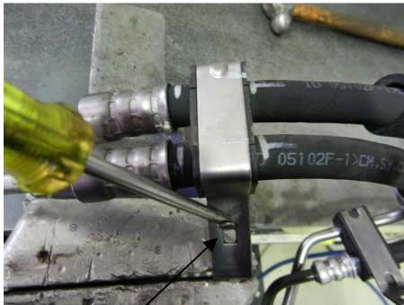
Using a screwdriver gently fold the steel tag open on the brackets. Take-care not to damage tag.
