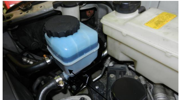
New "Modified" Bracket welded and bolted back into place on the vehicle.
