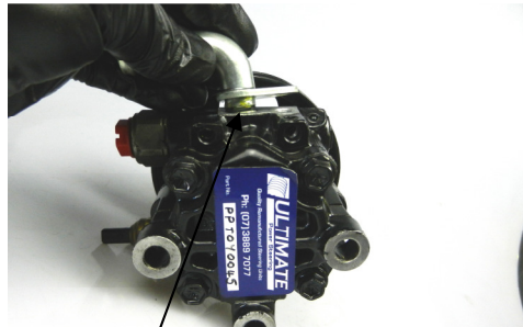
Photo 2 - New O-Ring installed onto fitting with small amount of grease on O-Ring for installation to pump housing.
