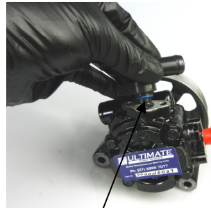
Photo 2 - New O-Ring installed onto fitting with small amount of grease on O-Ring for installation to pump housing.
