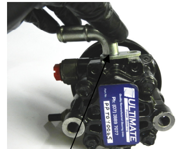
Photo 3 - New O-Ring installed on fitting and fitting bolted to Pump Housing ready for installation to vehicle.
