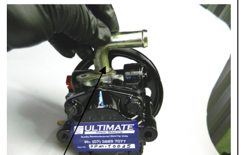
Photo 3 - New O-Ring installed on fitting and fitting bolted to Pump Housing ready for installation to vehicle.
