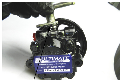
Photo 2 - New O-Ring installed onto fitting with small amount of grease on O-Ring for installation to pump housing.
