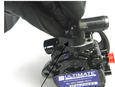
Photo 3 - New O-Ring installed on fitting and fitting bolted to Pump Housing ready for installation to vehicle.
