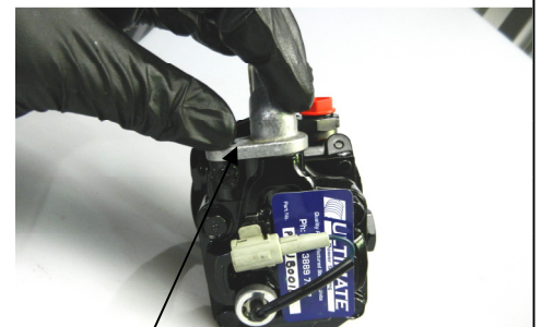
Photo 3 - New O-Ring installed on fitting and fitting bolted to Pump Housing ready for installation to vehicle.
